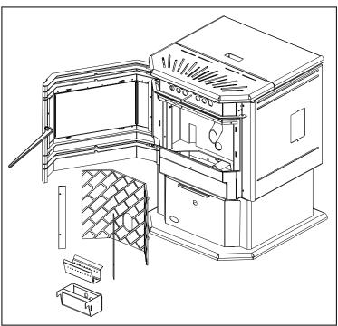
Figure 11: Firebox Components Removal.
